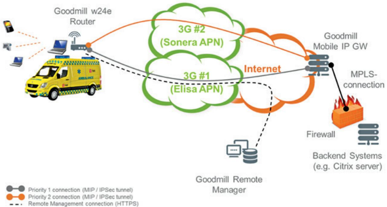
The figure shows that the hospital or command center can be connected to any vehicle through secured IPSec based VPNs through a VPN gateway. This VPN gateway can be any of the currently commercially available standard gateways. In case of high-end video surveillance, a special mobile IP server is needed on-site. This enables near seamless switching between networks with very little influence on picture quality or disruption to the video feed.
